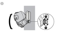
The default angle of the wall mount bracket is 90 degrees. You can maximize your baby unit's viewing angles by tilting the wall mount bracket.
